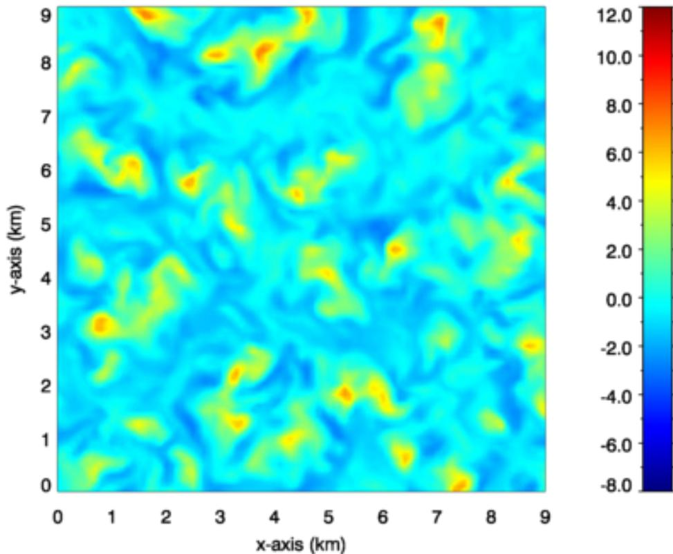
**Figure 2 – Vertical wind speed 1km above the Meridiani Terra surface, at local time 11:00. Results from a LMD mesoscale model simulation with 100m horizontal resolution (Large-Eddy Simulations). The model shows updrafts and downdrafts organizing according to a polygonal cellular structure as a result of the boundary layer turbulence. Note that the simulation was carried out without background wind.**
