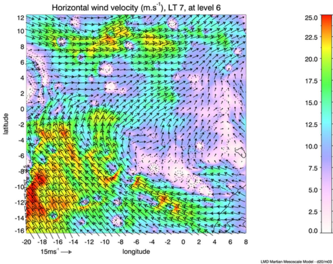
**Figure 1 - Horizontal wind speeds and vectors 520m above the Meridiani Terra surface, at local time 07:00. Results from a LMD mesoscale model simulation with 10km horizontal resolution. The model shows how moosoon and western boundary currents (large-scale meteorological circulations) are amplified by the local topography. Areas in red show strong horizontal winds: this information can be used to better constrain ExoMars landing design.**
