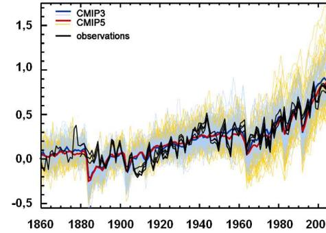
Mean surface temperature anomalies **observed** and **computed** considering *both the natural and anthropogenic perturbations* (observed volcanic eruptions and changes of the solar activity, the green house gases, the aerosols...)
