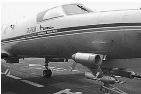
FIG. 2. Photograph of the AUSAT mounted under the fuselage of the Merlin IV after 1997.
