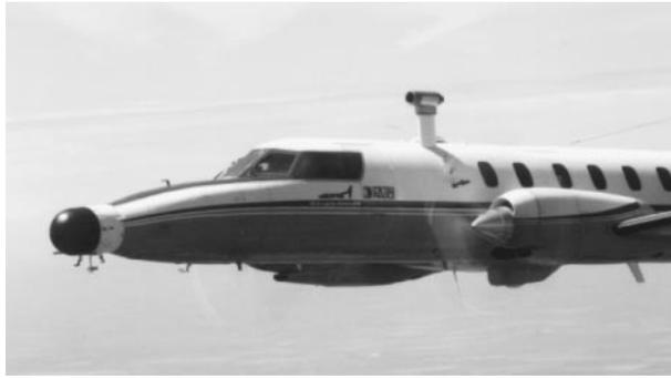
FIG. 1. Photograph of the AUSAT mounted above the fuselage of the Merlin IV in 1996.
