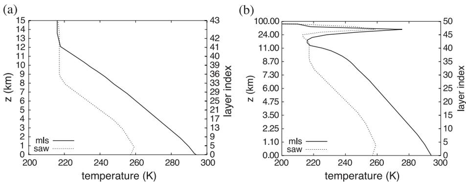
Fig. 4. Temperature profiles (K) in a McClatchey Mid-Latitude Summer (MLS) atmosphere and in a Sub-Arctic Winter (SAW) atmosphere. Scale is (a) linear with altitude and (b) linear with layer index.
