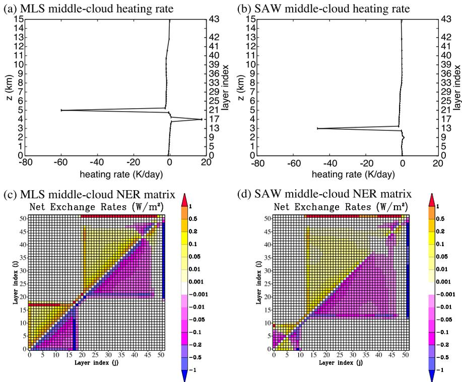
Fig. 7. (a) Heating rate ( $K/day$ ) for MLS middle-cloud configuration (water cloud extending from 4.0 to 5.0 km (layers 17–21) with  $LWC=0.28 \text{ g m}^{-3}$  and  $r_c=6.20 \text{ }\mu\text{m}$ ); (b) same as (a) for SAW atmosphere (water cloud extending from 2.0 to 3.0 km (layers 8–13) and same  $LWC$  and  $r_c$ ); (c) NER matrix  $W/m^2$  in the middle-cloud configuration for an MLS atmospheric profile; (d) same as (c) for a SAW atmospheric profile.
