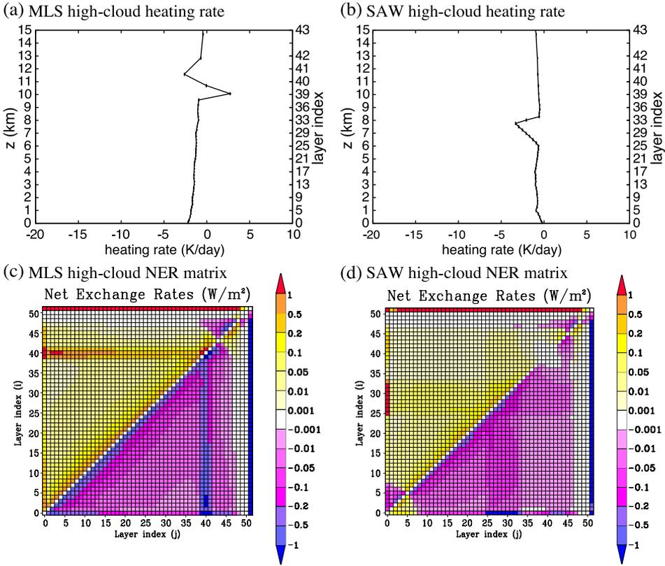
Fig. 8. (a) Heating rate ( $K/day$ ) for MLS high-cloud configuration (ice cloud extending from 10.0 to 12.0 km (layers 39–41) with  $IWC = 0.0048 \text{ g m}^{-3}$  and  $D_c = 41.5 \mu\text{m}$ ); (b) same as (a) for SAW atmosphere (water cloud extending from 6.0 to 8.0 km (layers 25–33) and same  $IWC$  and  $D_c$ ); (c) NER matrix ( $W/m^2$ ) in the high-cloud configuration for an MLS atmospheric profile; (d) same as (c) for a SAW atmospheric profile.
