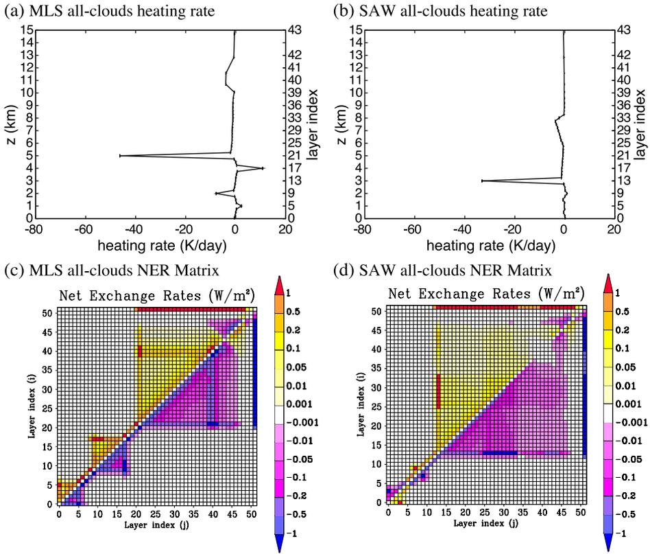
Fig. 9. (a) Heating rate (K/day) for MLS all-clouds configuration; (b) same as (a) for SAW atmosphere; (c) NER matrix ( $W/m^2$ ) for an MLS all-clouds configuration; (d) same as (c), for a SAW atmosphere.
