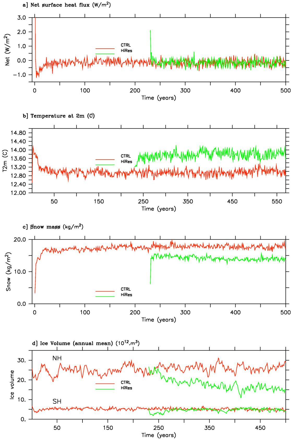
**Fig. 2** Evolution of global and annual averages of a) net surface heat flux ( $W m^{-2}$ ), b) temperature at 2 m (C), c) snow mass ( $kg m^{-2}$ ). D) ice volume ( $10^{12} m^3$ ) for Southern hemisphere (SH) and Northern hemisphere. Red for CTRL and green for HiRes
