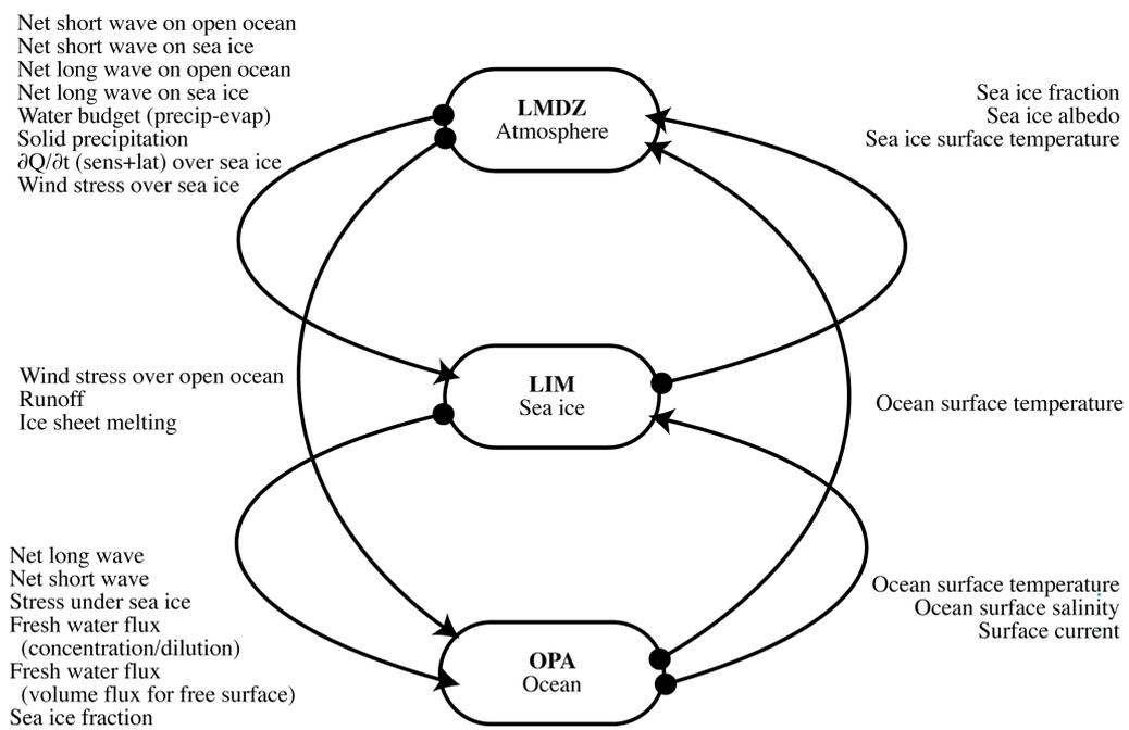
Fig. 1 Fields exchanged between ocean, sea ice and atmosphere models.
