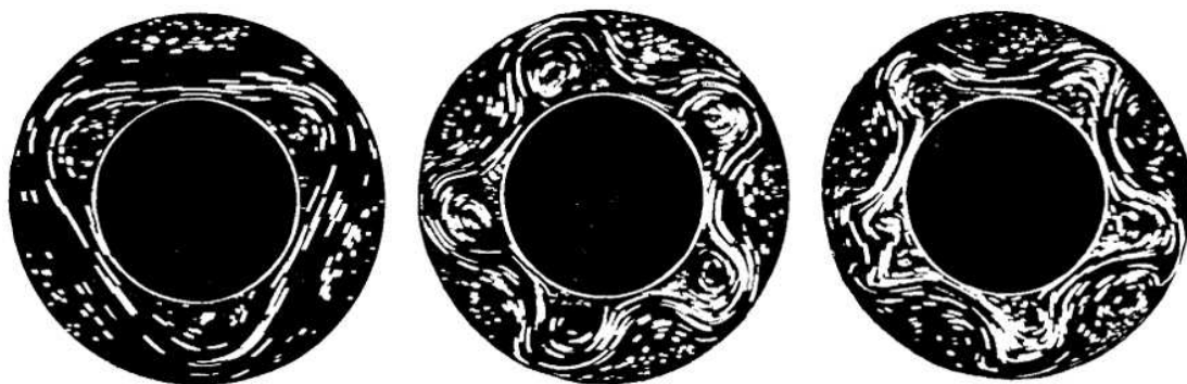
Figure 2.10: Rotating fluid with imposed temperature gradient. The rotation rate is increasing toward the right. From [Hide and Mason, 1975]
