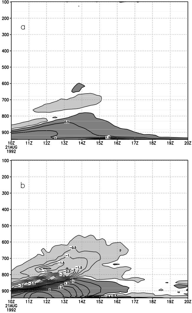
FIG. 1. HAPEX 92: August 21st squall line; prescribed heat source  $Q_1^{bl}/C_p$  (a) and moisture sink  $Q_2^{bl}/C_p$  (b) due to boundary layer processes ( $\text{K h}^{-1}$ ). Light gray and dark gray areas correspond to values below  $-0.1 \text{ K h}^{-1}$  and above  $0.1 \text{ K h}^{-1}$  respectively; contour spacing within these areas is  $0.5 \text{ K h}^{-1}$
