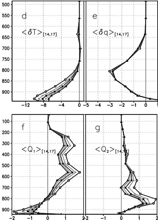
FIG. 14. HAPEX 92; August 21st squall line; time series of precipitation (a), wake height (b), and  $\sigma_w$  (c); vertical profiles of average values between 1400LT and 1700LT of  $\delta\theta$  (d),  $\delta q_v$  (e),  $Q_1/C_p$  (f), and  $Q_2/C_p$  (g) simulated by the SCM for various values of the tunable coefficient  $k_{gw}$ :  $k_{gw} = 0.5, 1., 1.5, 2., 2.5$  (curves with black open circles, gray closed circles, black closed squares, gray crosses, and black triangles respectively)
