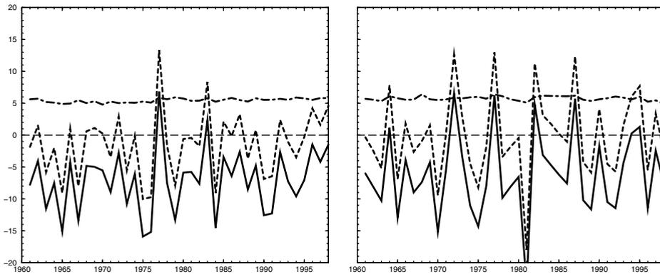
Figure 130: Time evolution of the Mediterranean Sea heat budget components (in  $\text{W/m}^2$ ) computed from the coupled simulation (left) and from the forced simulation (right). The surface heat flux is plotted in solid line, the Gibraltar heat transport in dashed line and the heat content change term in dotted line.
