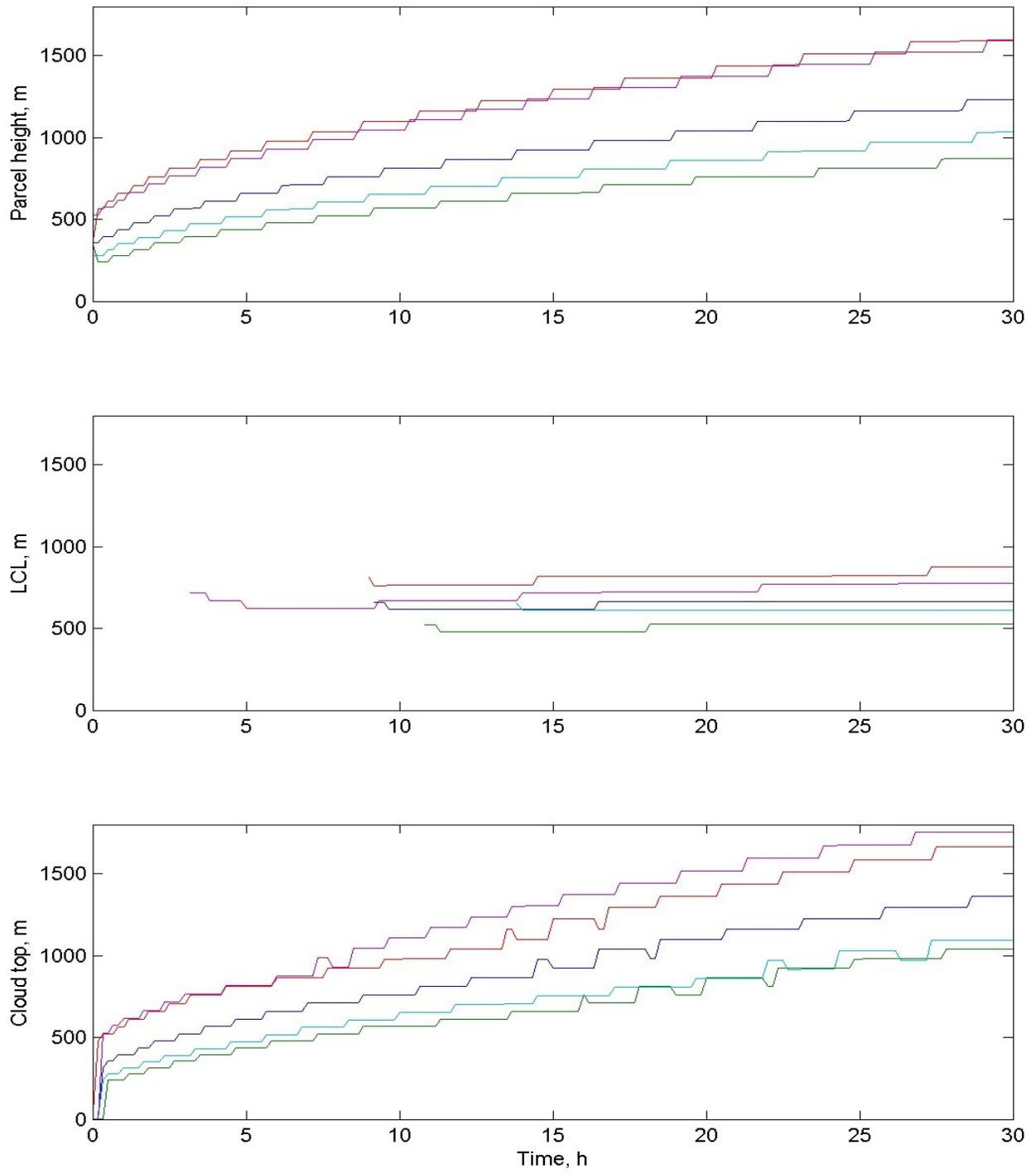
Example Figure 3: Parcel method BL height, lifting condensation level, and cloud top for the five STE runs with WRF-TEMF. Blue = run 1, green = 2, red = 3, cyan = 4, magenta = 5.
