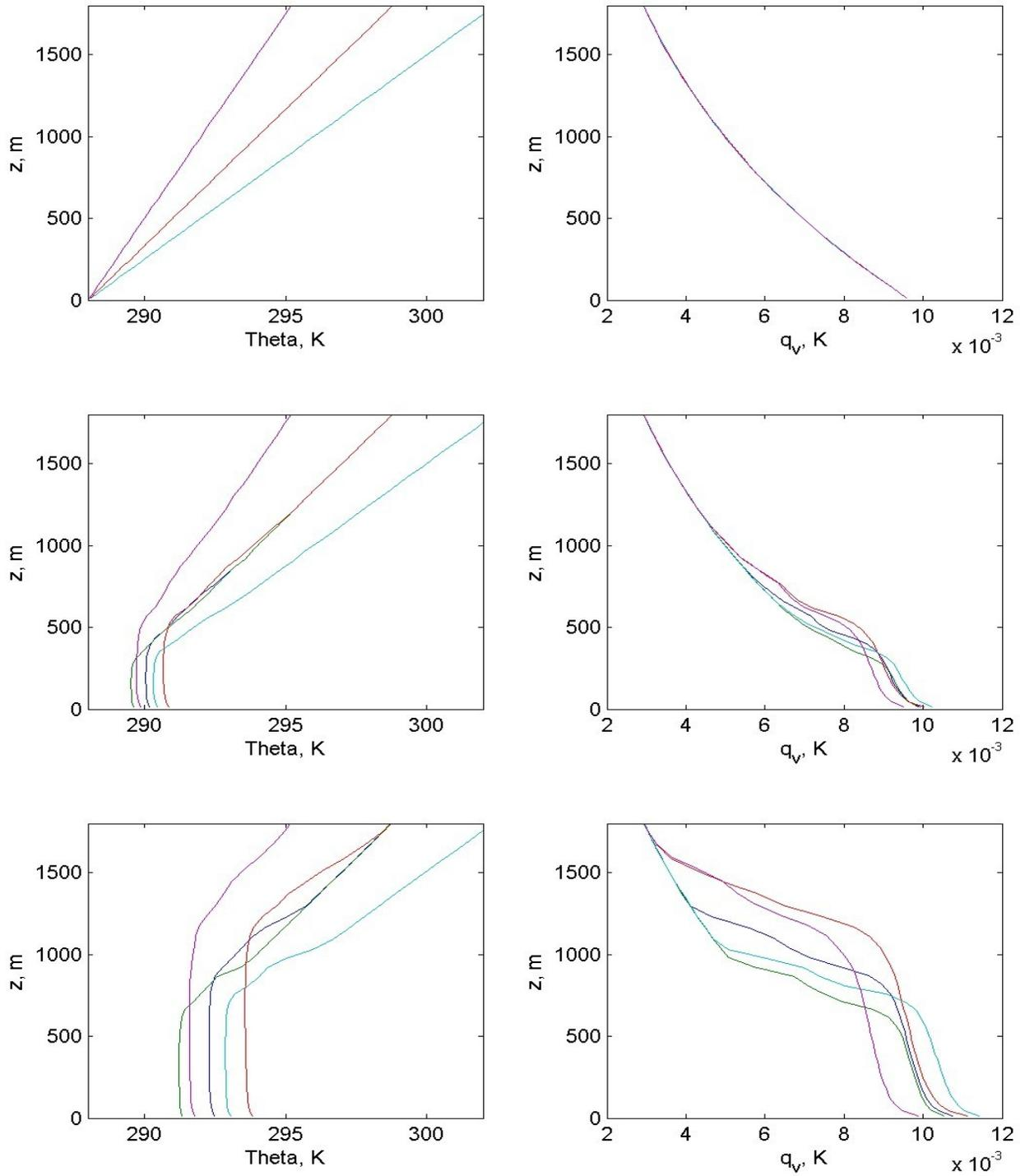
Example Figure 2: Potential temperature and water vapor profiles at times 0, 24000, and 96000 s for the five STE runs with WRF-TEMF. Blue = run 1, green = 2, red = 3, cyan = 4, magenta = 5.
