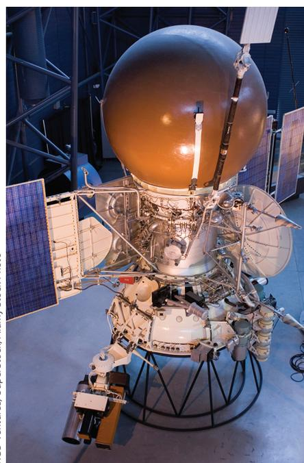
**Figure 2 | The VeGa-2 spacecraft.** Model of the spacecraft (located in the Steven F. Udvar-Házy Center, Dulles International Airport, Chantilly, Virginia, USA). The lander is hidden in the spherical shell on top of the spacecraft.
